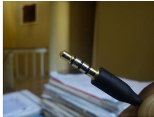
1/8 inch TRRS (3 pole mini) phone/headset cable (tip/ring/ring/sleeve)
